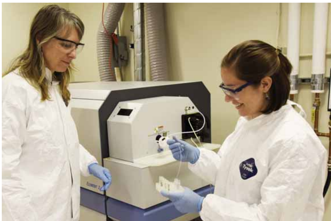
Ingrid Hendy (Professor) and Angela Dial injecting sample into new ELEMENT High Resolution ICP-MS. This instrument is capable of measurements of elemental concentration in the parts per trillion to quadrillion levels. Also available in the facility is a quadrupole mass spectrometer for rapid determination of elemental analysis at higher concentrations. Photo by Dale Austin.
