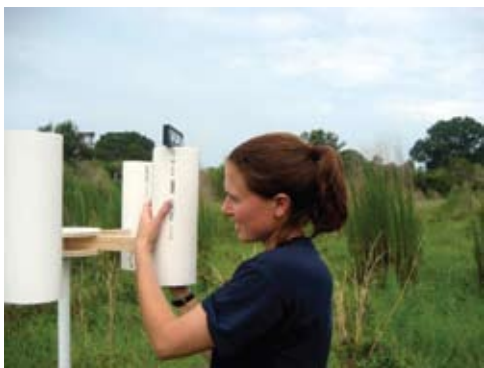
Laura Sherman (PhD candidate) setting up tripods to collect precipitation for research on mercury deposition in central Florida.
