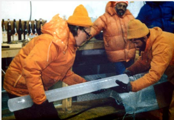
Removing ice core from core barrel at Dye-3, Greenland during GISP, 1980. Final depth of coring at this site was 2037 meters.
