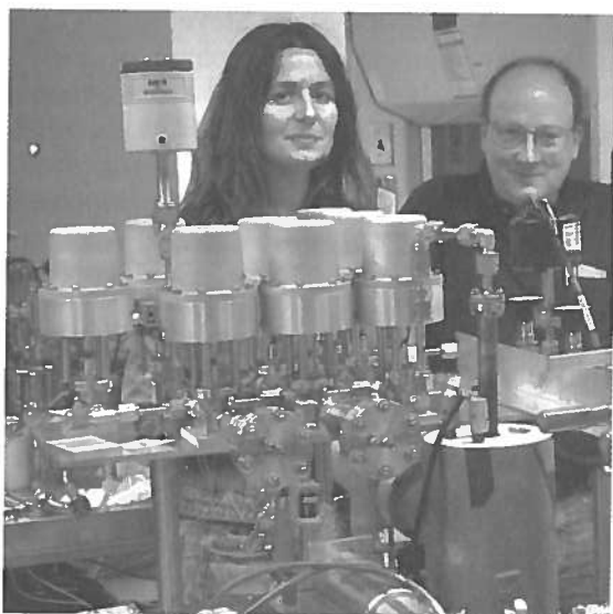
Construction of the extraction line in the Noble Gas Laboratory of the University of Michigan under the direction of Dr. Clara Castro. This highly innovative design is being developed with the collaboration of Dr. Chris Hall. Unlike most systems, this design has reduced the the total size of the system to less than one tenth of the current lines in operation at Lamont or ETH.
